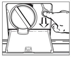
■ Pull the emergency release downwards (see illustration). The drum door will open.
